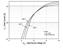
Figure 2. Transfer Characteristics
