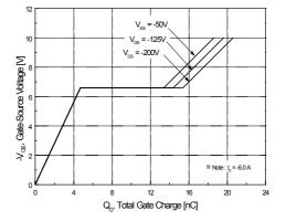
Figure 6. Gate Charge Characteristics
