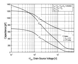
Figure 5. Capacitance Characteristics
