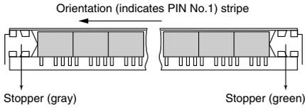
2) Tape and reel packing (surface-mount terminal type)
