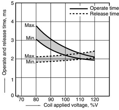
6-(2). Operate and release time (without diode)
