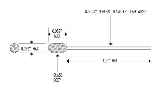
RESISTANCE @  $+25^{\circ}C$  =  $100,000 \Omega$  ± 10% RESISTANCE/TEMPERATURE CURVE = "L1" BETA " $\beta$ " (+25 TO  $+85^{\circ}C$ ) =  $4,040^{\circ}K$  NOMINAL TEMPERATURE COEFFICIENT @  $+25^{\circ}C$  = -4.52%/°C NOMINAL DISSIPATION CONSTANT = 0.45 mW/°C NOMINAL (AIR) THERMAL TIME CONSTANT = 2.5 SECONDS NOMINAL (AIR) MAXIMUM TEMPERATURE RATING =  $+300^{\circ}C$
