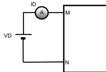
Figure 21. Test circuit for ID
