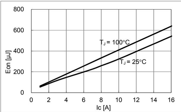
Figure 6.  $E_{ON}$  versus  $I_D$  for different temperatures
