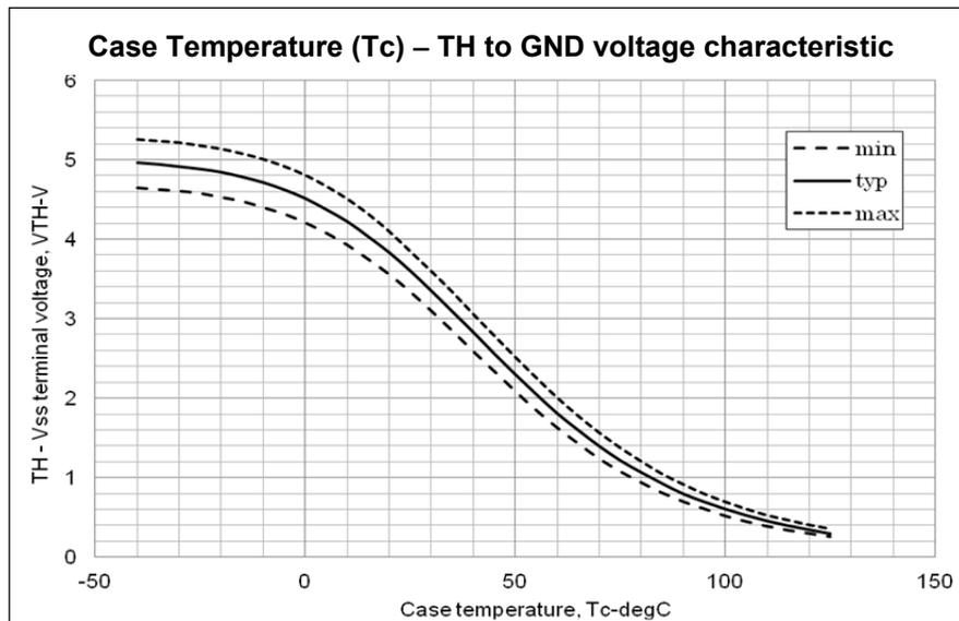
Figure 14. Thermistor Voltage versus Case Temperature
