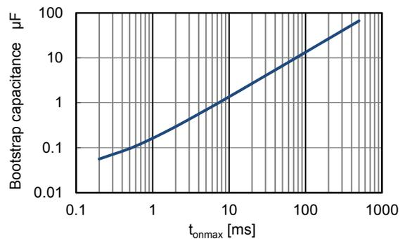
Figure 15. Bootstrap capacitance versus t<sub>ONMAX</sub>
