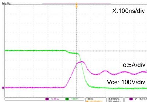
Figure 10. Turn-on waveform  $T_J = 100^\circ\text{C}$ ,  $V_{CC} = 400\text{ V}$
