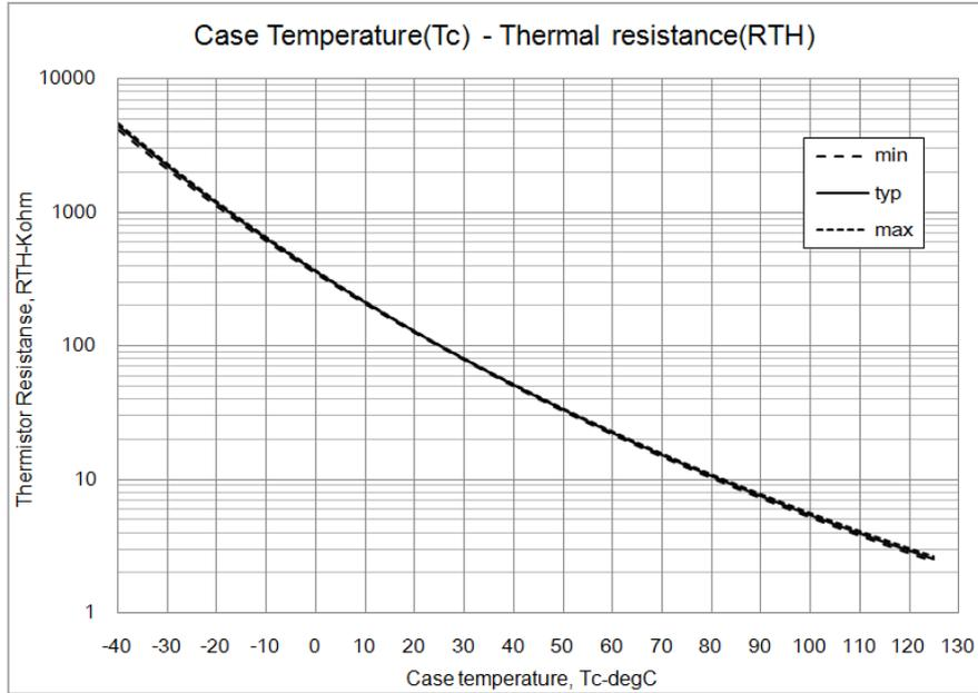
Figure13. Thermistor Resistance versus Case Temperature
