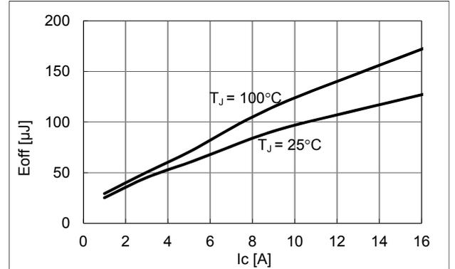
Figure 7.  $E_{OFF}$  versus  $I_D$  for different temperatures
