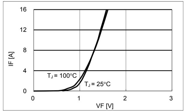
Figure 5.  $V_F$  versus  $I_D$  for different temperatures
