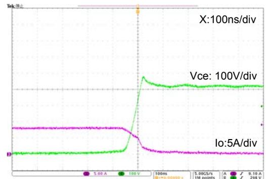
Figure 11. Turn-off waveform  $T_J = 100^\circ\text{C}$ ,  $V_{CC} = 400\text{ V}$
