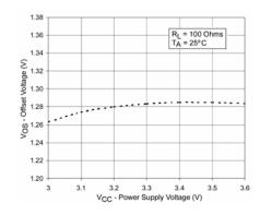
Figure 11.Offset Voltage vs. Power Supply Voltage
