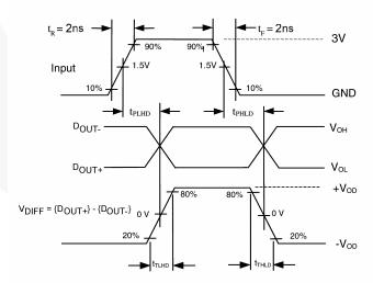
Figure 5. AC Waveforms
