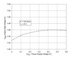
Figure 6. Output High Voltage vs. Power Supply Voltage
