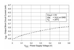
Figure 8. Output Short Circuit Current vs.
