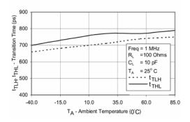
Figure 20. Transition Time vs. Ambient Temperature
