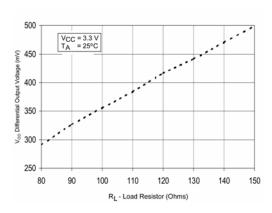
Figure 10.Differential Output Voltage vs. Load Resistor
