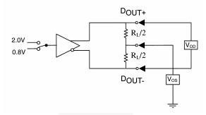
Figure 3. Differential Driver DC Test Circuit
