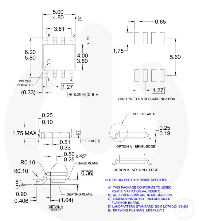
Figure 21.8-Lead Small Outline Integrated Circuit (SOIC), JEDEC MS-012, 0.150inch Narrow
