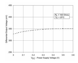
Figure 9. Differential Output Voltage vs. Power Supply Voltage
