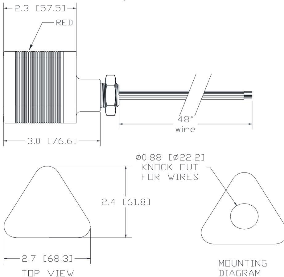
**LED OPERATION:** CONNECT STACK COLOR WIRE TO POWER AND BROWN WIRE TO POWER.
