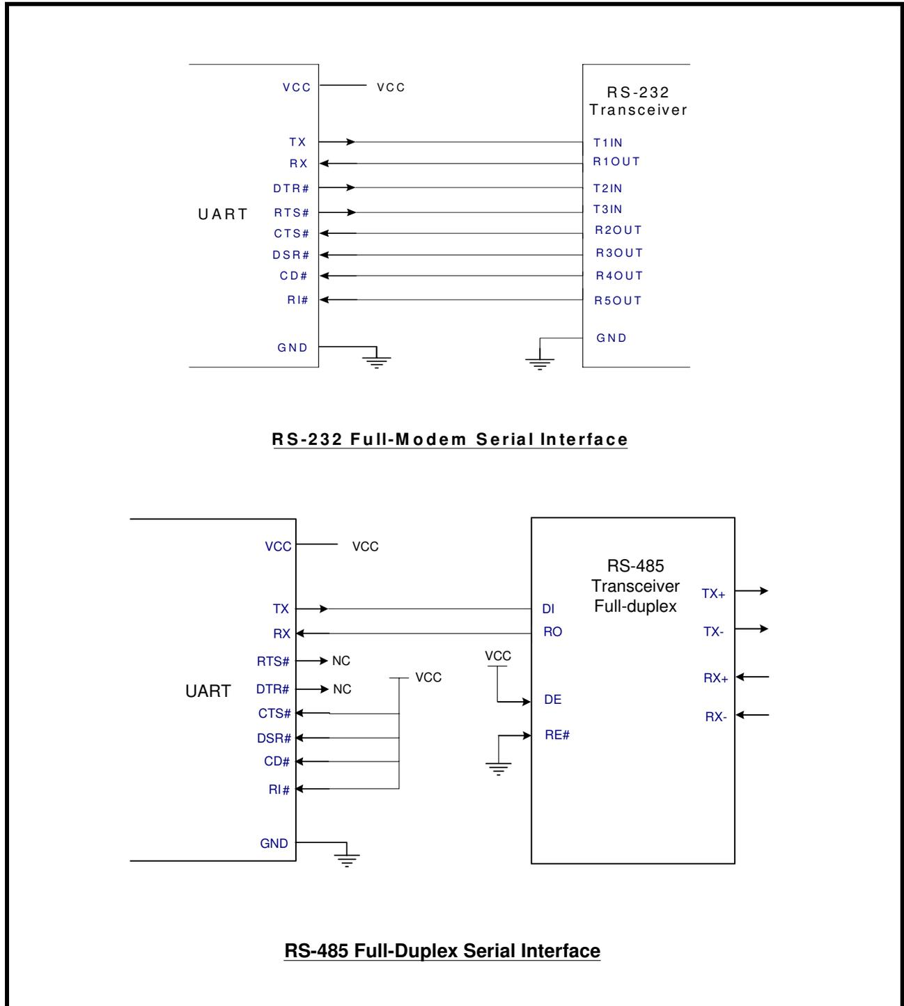
**FIGURE 5. XR16M570 TYPICAL SERIAL INTERFACE CONNECTIONS**
