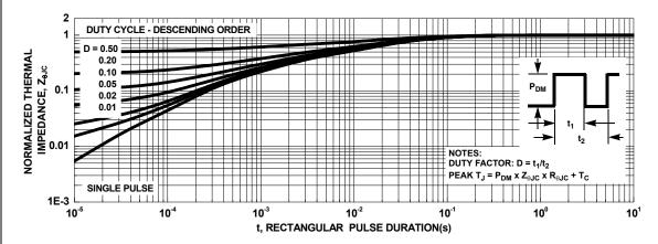
Figure 3. Normalized Maximum Transient Thermal Impedance
