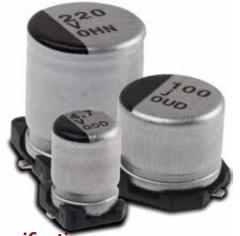
Type AVEK Capacitors are rated for 5000 hours at 105 °C with low impedance characteristics. They are ideal for high density PC board packaging. The Type AVEK offers a low in-place-cost for a high quality performer. The vertical cylindrical cases facilitate automatic mounting and reflow soldering into the same footprint of like-rated tantalum capacitors except without the need for voltage derating. Type AVEK is RoHS compliant.
