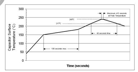
Case sizes 4 thur 6.3 mm dia. should be subjected to just one reflow soldering process. The 8 and 10 mm dia. case sizes should be subjected to a maximum of two reflow soldering processes.
