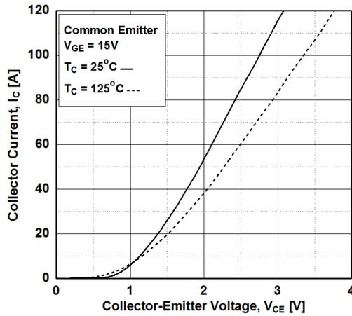
Figure 4. Transfer Characteristics
