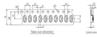
Taping condition: Lack of products in the middle of taping should be one MAX, but total quantity specified in the specifications should be secured.
