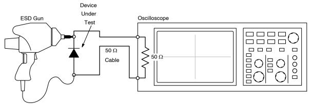
Figure 4. Diagram of ESD Test Setup
