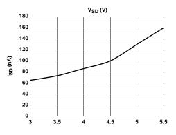
FIGURE 2. DIGITAL SUPPLY CURRENT vs DIGITAL SUPPLY VOLTAGE
