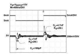
FIGURE 4. TRANSIENT LOAD REGULATION (SOURCING)
