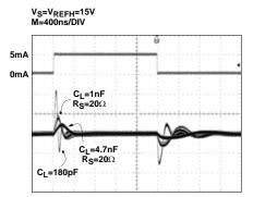
FIGURE 5. TRANSIENT LOAD REGULATION (SINKING)
