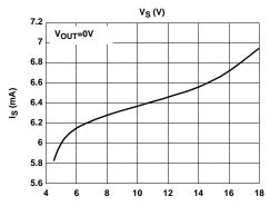
FIGURE 3. SUPPLY CURRENT vs SUPPLY VOLTAGE
