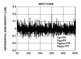
FIGURE 1. DIFFERENTIAL NONLINEARITY vs CODE
