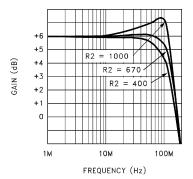
FIGURE 2. FREQUENCY RESPONSE vs RESISTOR R2 (GAIN = 2)
