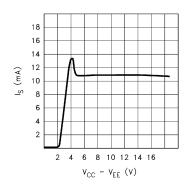
FIGURE 1. IS vs SUPPLY VOLTAGE
