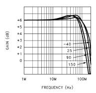
FIGURE 3. FREQUENCY RESPONSE vs TEMPERATURE
