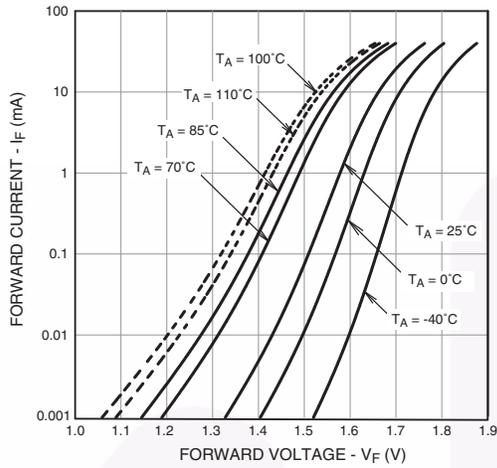
Fig. 6 LED Forward Current vs. Forward Voltage
