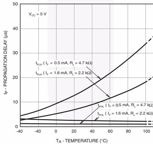
Fig. 14 Propagation Delay vs. Temperature (6N138M / 6N139M Only)
