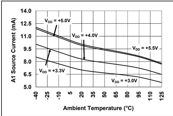
**FIGURE 2-14:** Amplifier A1 Source Current vs. Temperature.
