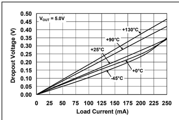
**FIGURE 2-32:** LDO Dropout Voltage vs. Load Current.
