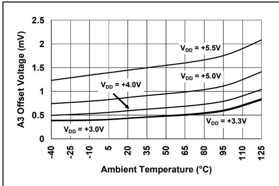
**FIGURE 2-19:** Amplifier A3 Offset Voltage vs. Temperature.
