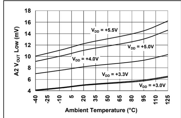
**FIGURE 2-16:** Amplifier A2 Output Voltage Low vs. Temperature.
