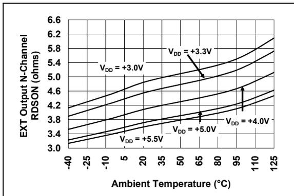
**FIGURE 2-8:**  $V_{EXT}$  N-Channel Driver  $R_{DSON}$  vs. Temperature.
