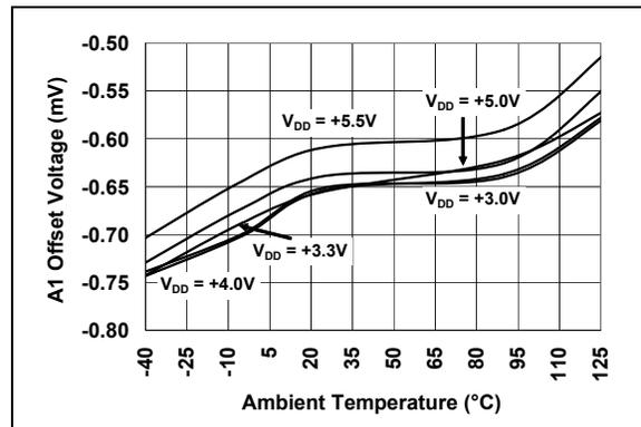
**FIGURE 2-11:** Amplifier A1 Offset Voltage vs. Temperature.
