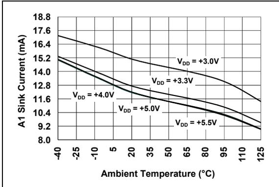
**FIGURE 2-13:** Amplifier A1 Sink Current vs. Temperature.
