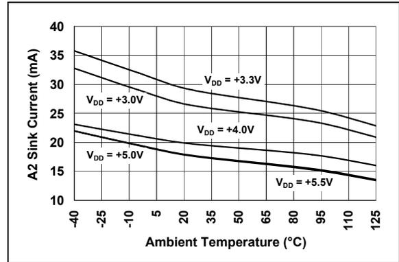
**FIGURE 2-17:** Amplifier A2 Sink Current vs. Temperature.
