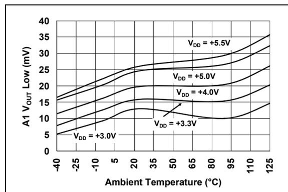
**FIGURE 2-12:** Amplifier A1 Output Voltage Low vs. Temperature.
