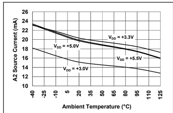
**FIGURE 2-18:** Amplifier A2 Source Current vs. Temperature.
