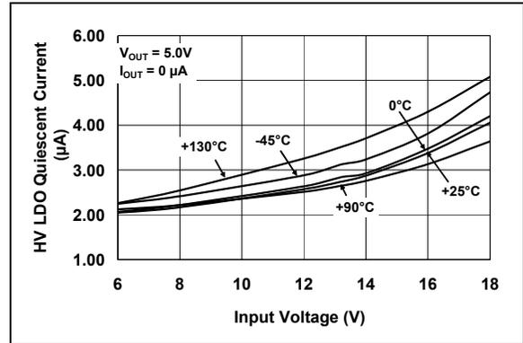
**FIGURE 2-29:** LDO Quiescent Current vs. Input Voltage.
