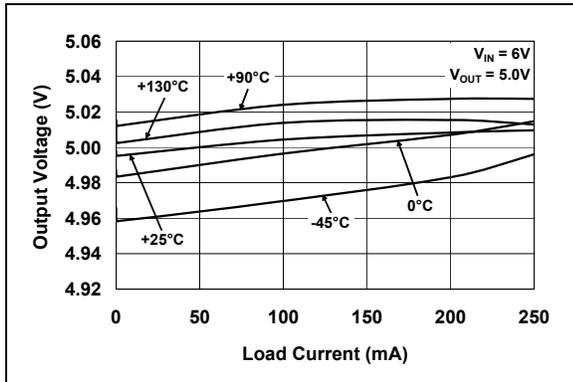
**FIGURE 2-31:** LDO Output Voltage vs. Load Current.
