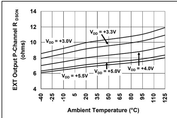
**FIGURE 2-7:**  $V_{EXT}$  P-Channel Driver  $R_{DSON}$  vs. Temperature.
