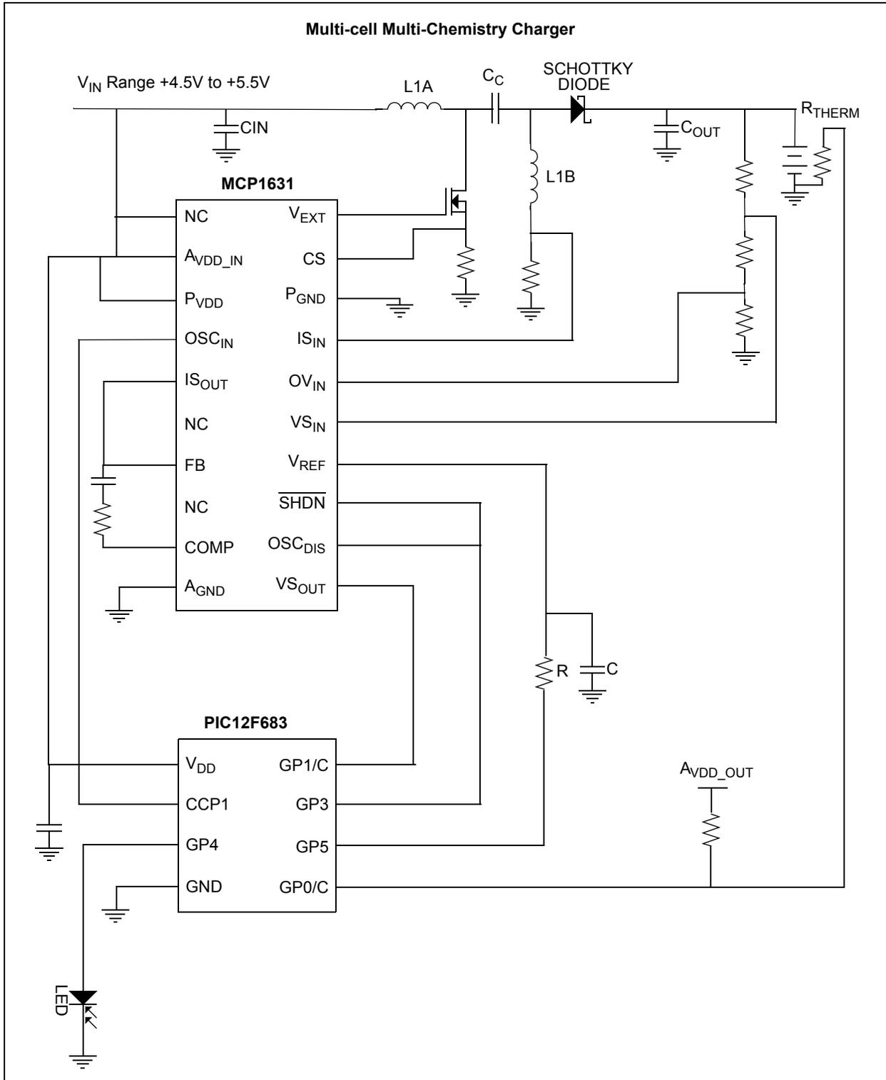
**FIGURE 5-1:** +5V ac-dc or USB Input Application.
