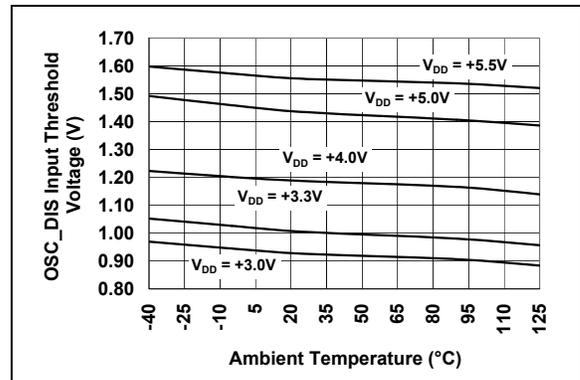
**FIGURE 2-6:** Oscillator Disable Input Threshold vs. Temperature.
