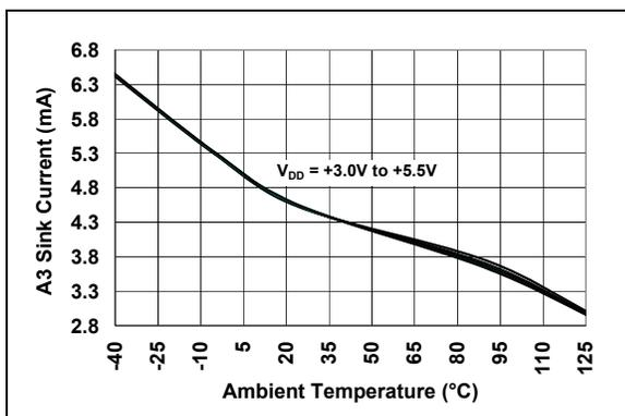
**FIGURE 2-21:** Amplifier A3 Sink Current vs. Temperature.
