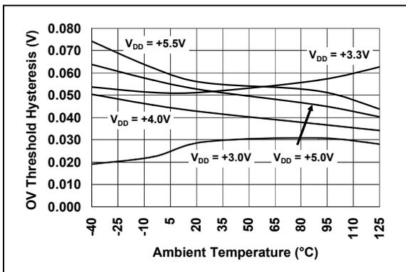
**FIGURE 2-27:** Overtolerance Threshold Hysteresis (V) vs. Temperature.
