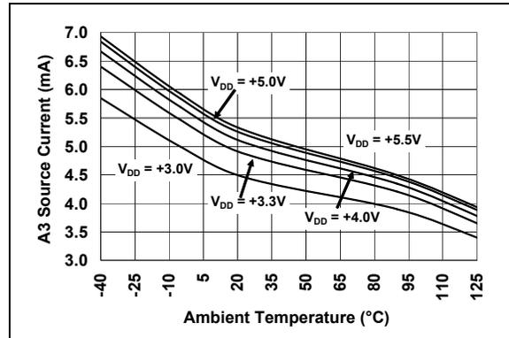
**FIGURE 2-22:** Amplifier A3 Source Current vs. Temperature.
