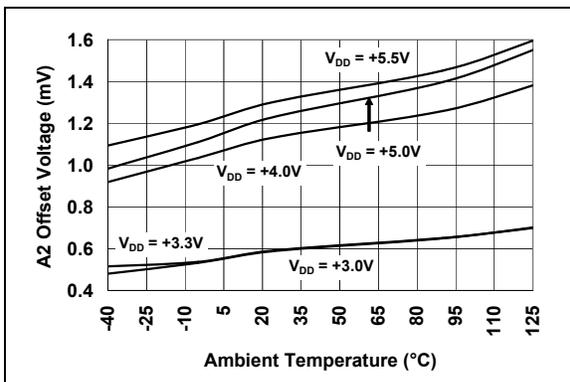
**FIGURE 2-15:** Amplifier A2 Offset Voltage vs. Temperature.
