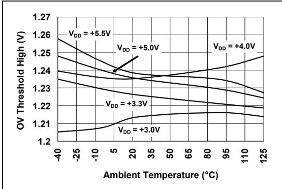
**FIGURE 2-25:** Overtolerance Threshold High (V) vs. Temperature.
