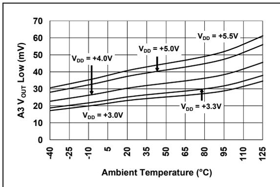
**FIGURE 2-20:** Amplifier A3 Output Voltage Low vs. Temperature.
