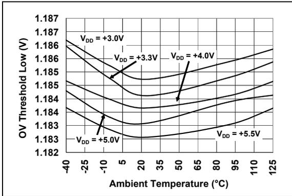
**FIGURE 2-26:** Overtolerance Threshold Low (V) vs. Temperature.
