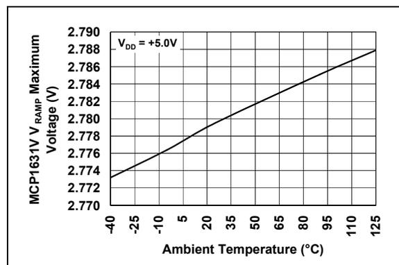
**FIGURE 2-24:** MCP1631V and MCP1631VHV  $V_{RAMP}$  Max Voltage (V).
