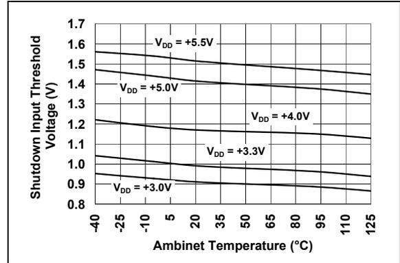
**FIGURE 2-28:** Shutdown Input Voltage Threshold (V) vs. Temperature.
