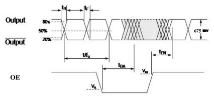
Figure 2. HCSL Output Waveform
