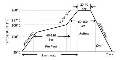
Figure 3. Solder Reflow Profile
