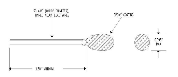
RESISTANCE @  $+25^{\circ}C = 3,000 \ \Omega$  NOMINAL ACCURACY (0 TO  $+70^{\circ}C$ ) =  $\pm$  0.10°C RESISTANCE/TEMPERATURE CURVE = "J" TEMPERATURE COEFFICIENT @  $+25^{\circ}C = -4.4\%$ /°C NOMINAL BETA " $\beta$ " (0 TO  $+50^{\circ}C$ ) = 3,892°K NOMINAL DISSIPATION CONSTANT = 1 mW/°C NOMINAL THERMAL TIME CONSTANT = 10 SECONDS MAXIMUM (STILL AIR) THERMAL TIME CONSTANT = 1 SECOND MAXIMUM (WELL STIRRED OIL) MAXIMUM TEMPERATURE RATING =  $+150^{\circ}C$
