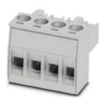
PCB connector, nominal current: 16 A, rated voltage (III/2): 320 V, number of positions: 4, pitch: 5 mm, connection method: Screw connection, color: light gray, contact surface: Tin
