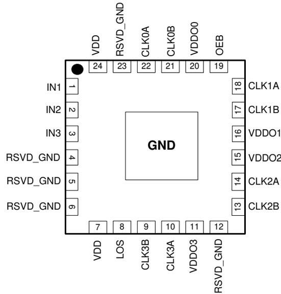
**Note:** Center pad must be tied to GND for normal operation.
