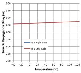
Figure 5. Turn-on Propagation Delay vs. Temperature
