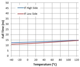
Figure 11. Fall Time vs. Temperature
