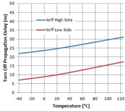
Figure 7. Turn-off Propagation Delay vs. Temperature
