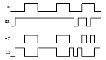
Figure 2. Input / Output Timing Diagram
