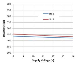
Figure 24. Deadtime vs. Supply Voltage
