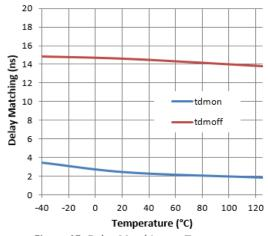
Figure 15. Delay Matching vs. Temperature
