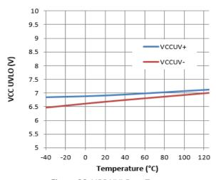
Figure 26. VCC UVLO vs. Temperature
