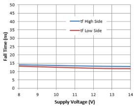
Figure 10. Fall Time vs. Supply Voltage
