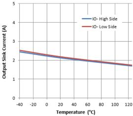
Figure 19. Output Sink Current vs. Temperature
