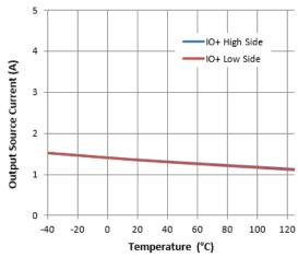
Figure 17. Output Source Current vs. Temperature
