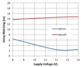
Figure 14. Delay Matching vs. Supply Voltage
