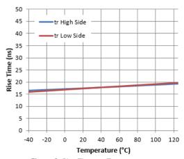
Figure 9. Rise Time vs. Temperature
