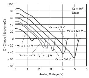
**Charge Injection vs. Analog Voltage**
