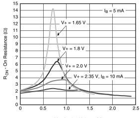
V<sub>A</sub> - Analog Voltage (V)
