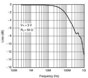
Insertion Loss vs. Frequency
