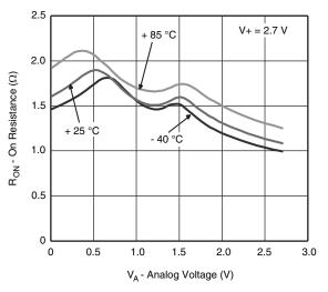
$R_{\text{ON}}$  vs.  $V_{\text{D}}$  and Temperature
