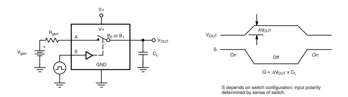
Fig. 3 - Charge Injection
