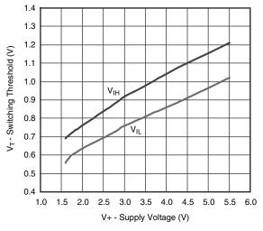
Switching Threshold vs. Supply Voltage
