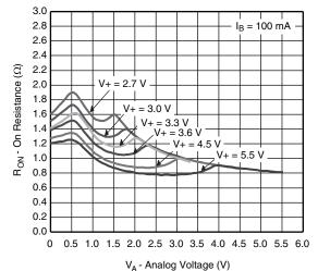
R<sub>ON</sub> vs. V<sub>A</sub> and Supply Voltage
