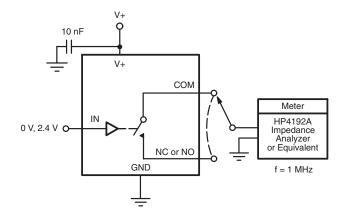
Figure 5. Channel Off/On Capacitance
