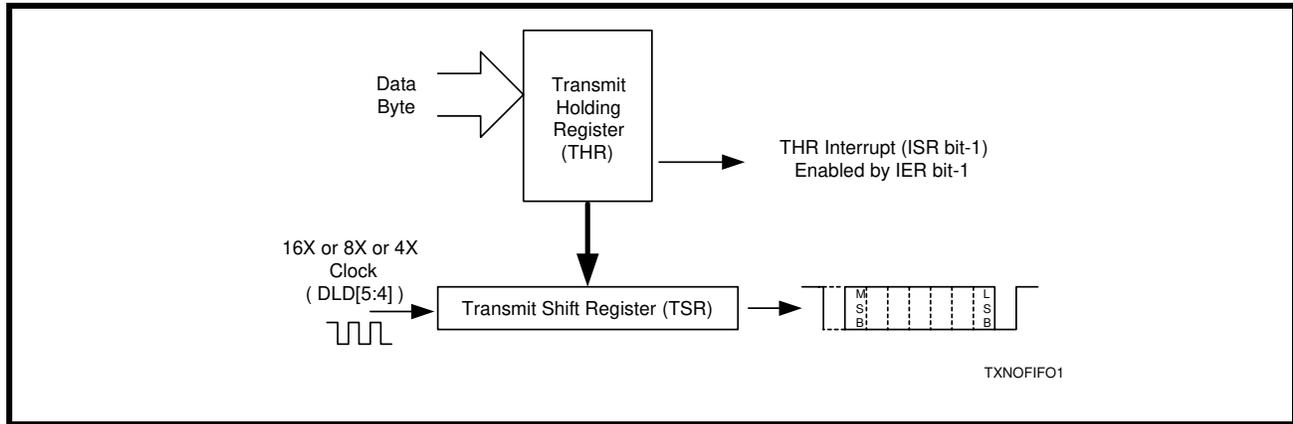
2.9.3 Transmitter Operation in FIFO Mode
