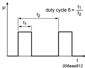
Fig. 17. Duty cycle definition
