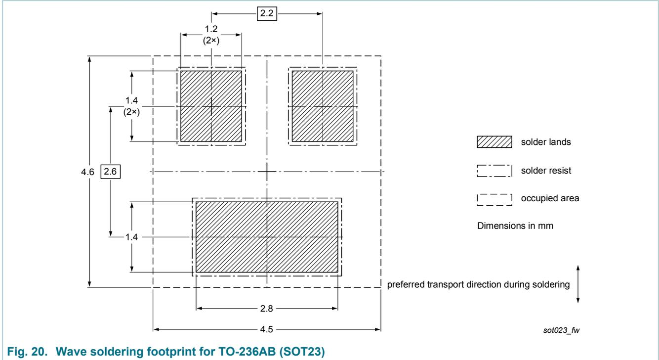
Fig. 20. Wave soldering footprint for TO-236AB (SOT23)
