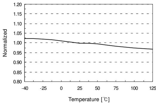
**Figure 8. Shutdown Feedback Voltage ( $V_{SD}$ ) vs.  $T_A$**
