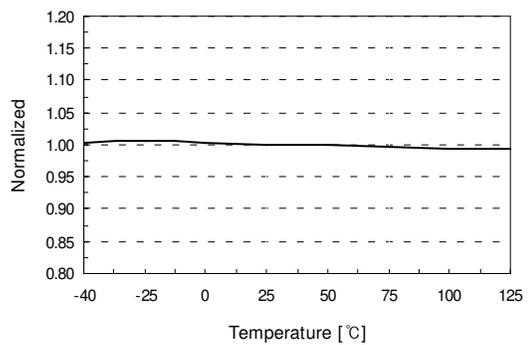
**Figure 9. Maximum Duty Cycle ( $D_{MAX}$ ) vs.  $T_A$**
