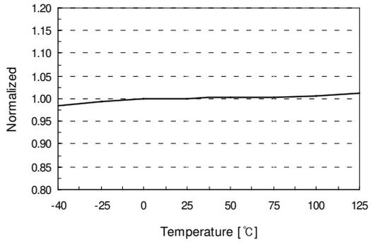
Figure 12. Operating Supply Current (I<sub>OP</sub>) vs. T<sub>A</sub>
