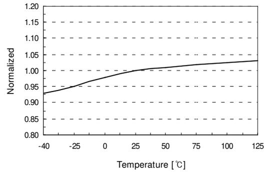
Figure 11. Shutdown Delay Current (I<sub>DELAY</sub>) vs. T<sub>A</sub>
