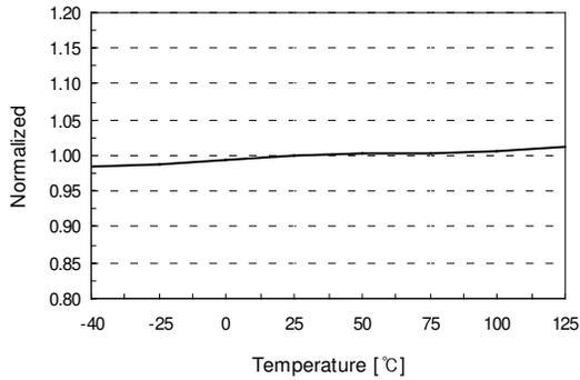
**Figure 6. Start Threshold Voltage ( $V_{START}$ ) vs.  $T_A$**
