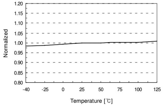
**Figure 7. Stop Threshold Voltage ( $V_{STOP}$ ) vs.  $T_A$**
