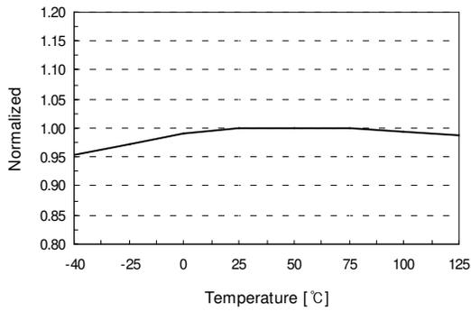
**Figure 4. Operating Frequency ( $f_{osc}$ ) vs.  $T_A$**
