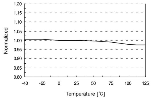
**Figure 5. Peak Current Limit ( $I_{LIM}$ ) vs.  $T_A$**
