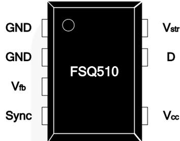
Figure 3. Pin Assignments
