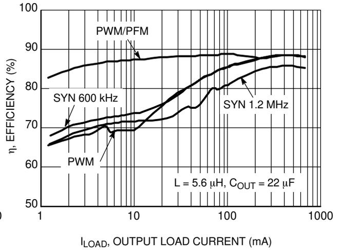
**Figure 22. Efficiency vs. Output Load Current**
