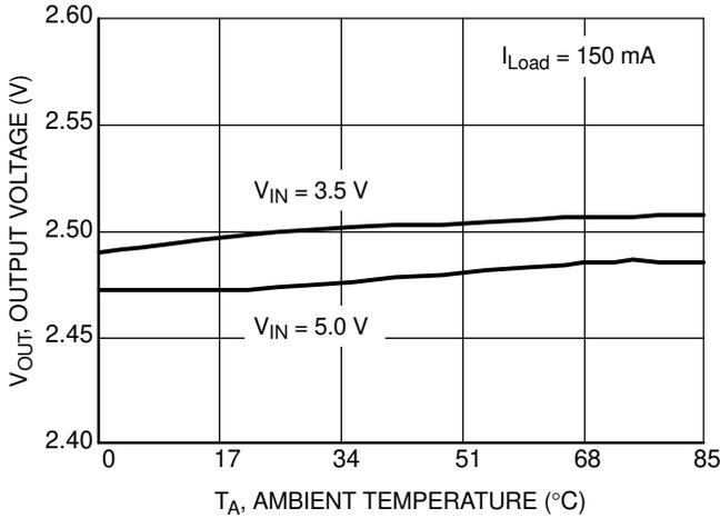
**Figure 3. Output Voltage vs. Ambient Temperature ( $V_{OUT} = 2.5$  V)**
