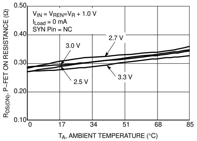
**Figure 10. P-FET ON Resistance vs. Ambient Temperature**
