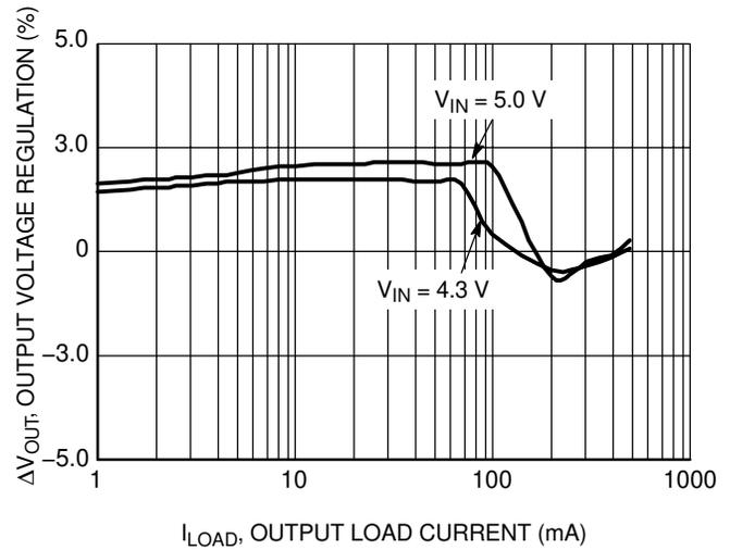
**Figure 26. Output Voltage Regulation vs. Output Load Current**
