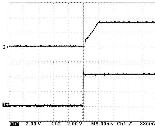
( $V_{IN} = 4.3\text{ V}$ ,  $V_{OUT} = 3.3\text{ V}$ ,  $C_{SS} = 100\text{ pF}$ , No load)
