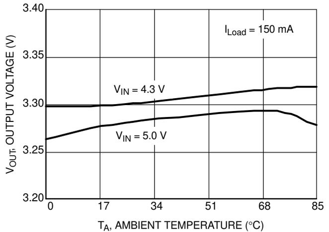
**Figure 6. Output Voltage vs. Ambient Temperature ( $V_{OUT} = 3.3$  V)**
