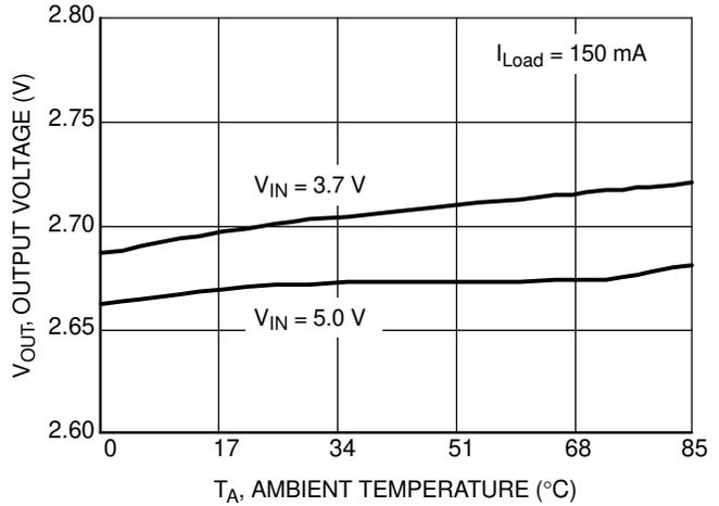
**Figure 4. Output Voltage vs. Ambient Temperature ( $V_{OUT} = 2.7$  V)**
