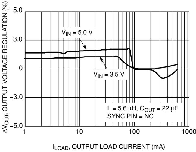
**Figure 23. Output Voltage Regulation vs. Output Load Current**
