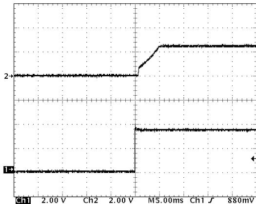
( $V_{IN} = 3.5\text{ V}$ ,  $V_{OUT} = 2.5\text{ V}$ ,  $C_{SS} = 100\text{ pF}$ , No load)
