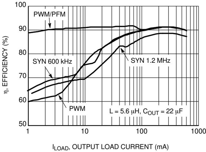
**Figure 21. Efficiency vs. Output Load Current**
