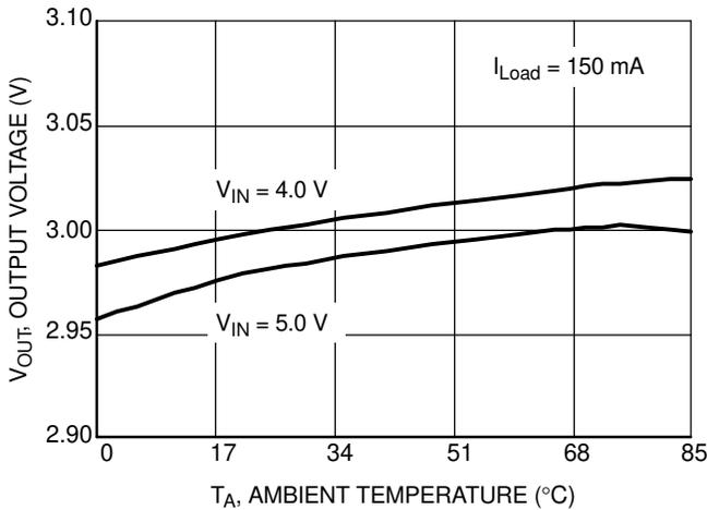
**Figure 5. Output Voltage vs. Ambient Temperature ( $V_{OUT} = 3.0$  V)**
