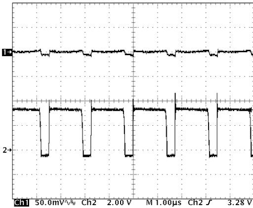
( $V_{IN} = 3.5\text{ V}$ ,  $V_{OUT} = 2.5\text{ V}$ ,  $I_{LOAD} = 600\text{ mA}$ )
