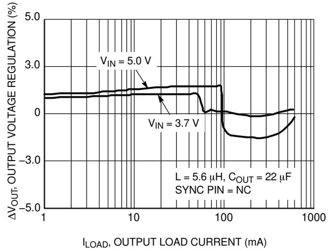
**Figure 24. Output Voltage Regulation vs. Output Load Current**
