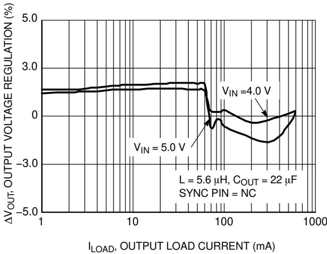
**Figure 25. Output Voltage Regulation vs. Output Load Current**
