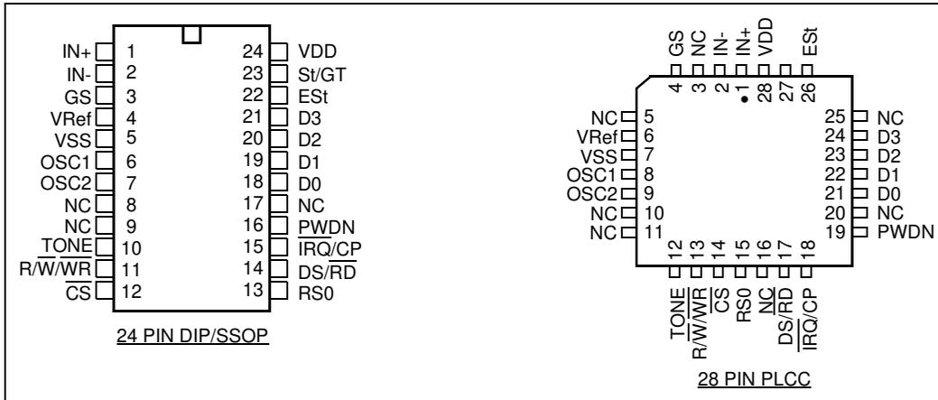
Figure 2 - Pin Connections
