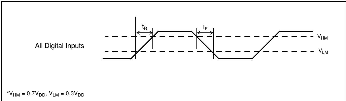
**Figure 15 - Digital Signal Input Rise/Fall Times**
