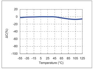
4) Bias TCC characteristics (Agilent 4284A, 1kHz, 1.0Vrms, 25Vdc)
