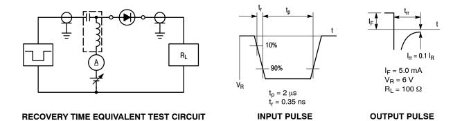
Figure 4. Reverse Recovery Time Test Circuit for the DAN222
