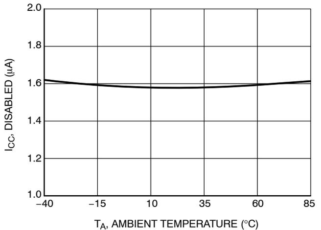
**Figure 8. Quiescent Current Into V<sub>CC</sub> vs. Temperature**
