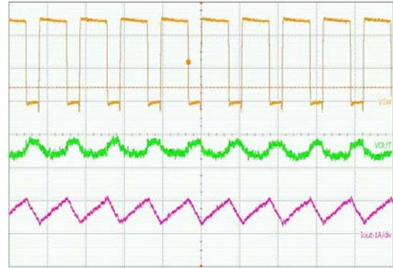
( $V_{IN} = 5\text{ V}$ ,  $I_{LOAD} = 700\text{ mA}$ ,  $L = 3.3\text{ }\mu\text{H}$ ,  $C_{OUT} = 2 \times 22\text{ }\mu\text{F}$ )
