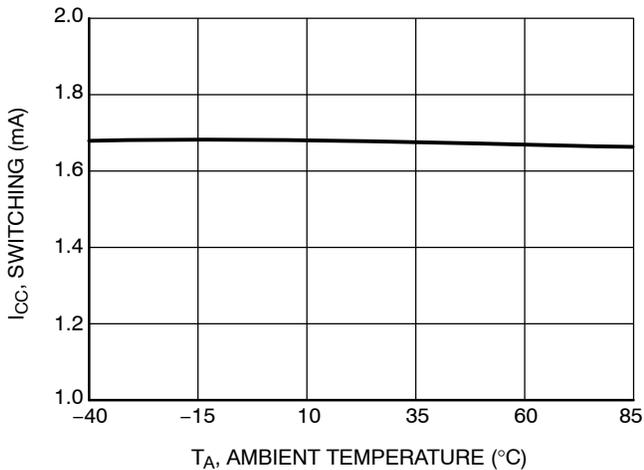
**Figure 7. Quiescent Current Into V<sub>CC</sub> vs. Temperature**
