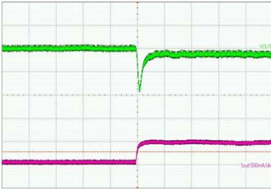
( $V_{IN} = 5\text{ V}$ ,  $I_{LOAD} = 100\text{ mA}$ ,  $L = 3.3\text{ }\mu\text{H}$ ,  $C_{OUT} = 2 \times 22\text{ }\mu\text{F}$ )
