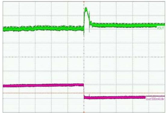
( $V_{IN} = 5\text{ V}$ ,  $I_{LOAD} = 100\text{ mA}$ ,  $L = 3.3\text{ }\mu\text{H}$ ,  $C_{OUT} = 2 \times 22\text{ }\mu\text{F}$ )
