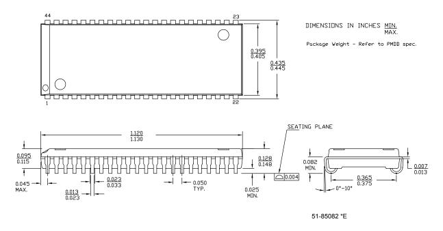
Figure 10. 44-pin TSOP II Package Outline, 51-85087
