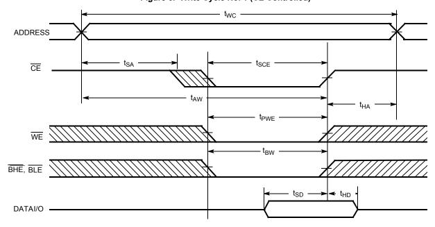
Figure 7. Write Cycle No. 2 (BLE or BHE Controlled)
