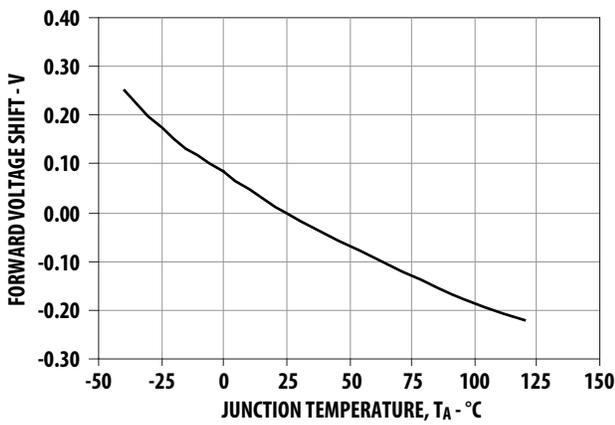
Figure 8. Relative forward voltage shift vs Temperature
