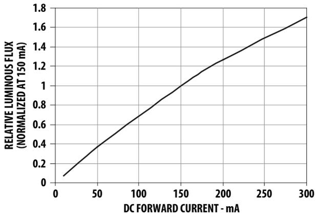
Figure 1. Relative luminous flux vs Forward current
