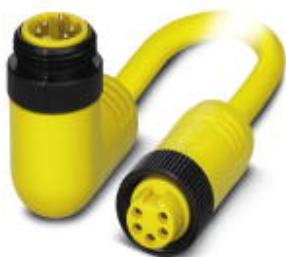
Power cable, 5-position, PVC, yellow, Plug angled 7/8"-16UNF, on Socket straight 7/8"-16UNF, cable length: 10 m
