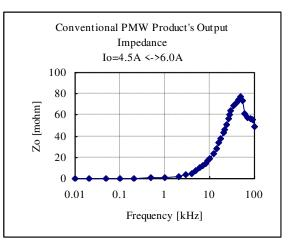
Fig. 12.2.2 Output Impedance of conventional product
