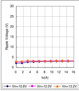
Fig. 12.3.3 Ripple Voltage v.s. Output Current
