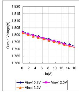
Fig. 12.3.1 Output Voltage v.s. Output Current
