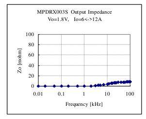
Fig. 12.2.1 Output Impedance of MPDRX003S
