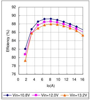
Fig. 12.3.2 Efficiency v.s. Output Current
