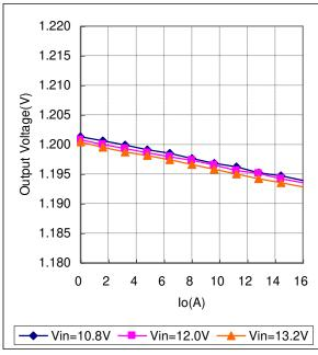
Fig. 12.3.4 Output Voltage v.s. Output Current
