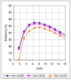
Fig. 12.3.5 Efficiency v.s. Output Current
