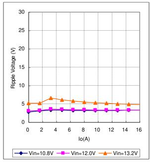
Fig. 12.3.6 Ripple Voltage v.s. Output Current
