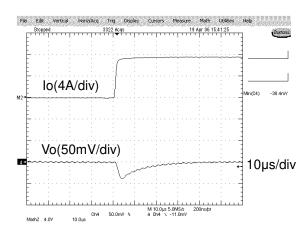
Fig. 12.1 Load Transient Response
