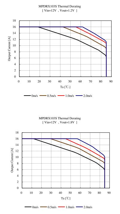
The above derating limits apply to this product soldered directly to 101.6\*180mm\*1.6mm PCB (double-sided, with 70um copper). Any adjacent parts of high temperature may cause overheating. For reliable operation, please ensure that the FET temperature of this product is maintained below 120°C and the inductor temperature is below 106°C.
