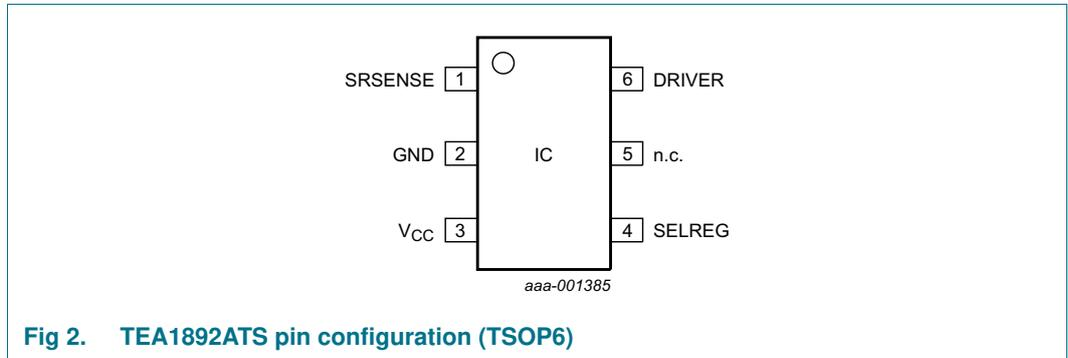
Fig 2. TEA1892ATS pin configuration (TSOP6)
