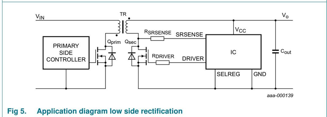
Fig 5. Application diagram low side rectification
