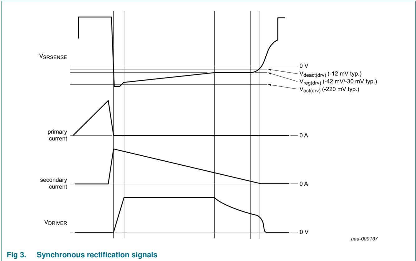
Fig 3. Synchronous rectification signals
