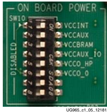
Figure 1-5: Core Power Regulator Enable Switches SW10
