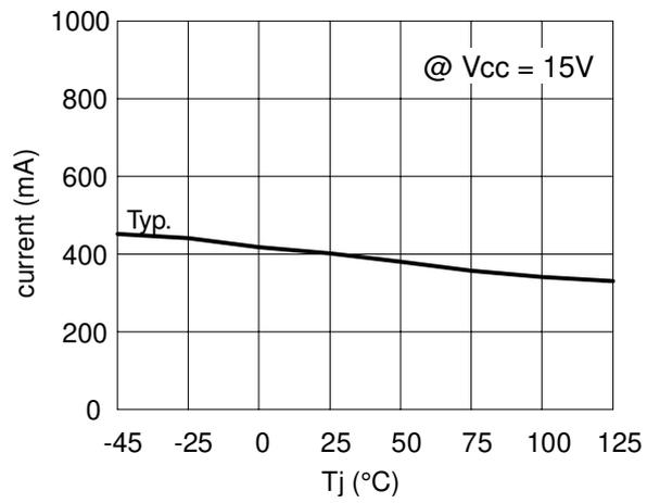
**Figure 7. Output Sink Current vs. Temperature**
