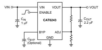
Figure 1. Application Schematic
