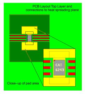
Figure 29. Topside Copper Foil Pattern for Heat Dissipation
