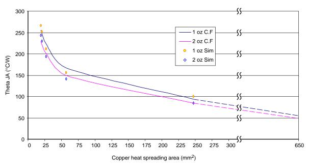
Figure 28. Thermal Resistance vs. PCB Copper Area for 3 mm x 3 mm WDFN Package
