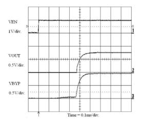
Figure 24. Enable Turn-On (1 mA Load)  $(V_{OUT} = 0.8 \text{ V and } V_{IN} = 1.8 \text{ V})$
