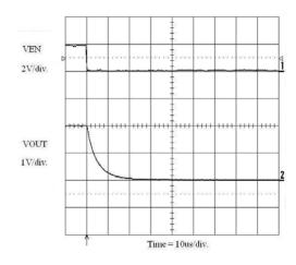
Figure 18. Enable Turn-Off (1000 mA Load)
