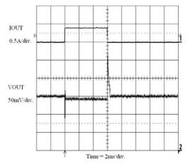
Figure 25. Load Transient Response (1 mA to 400 mA) ( $V_{OUT}$  = 0.8 V and  $V_{IN}$  = 1.8 V)
