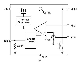
Figure 2. Simplified Block Diagram
