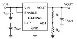
Figure 27. Adjustable Output Resistor Divider
