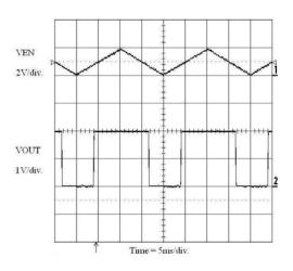
Figure 22. Slow Enable Operation (1000 mA Load)
