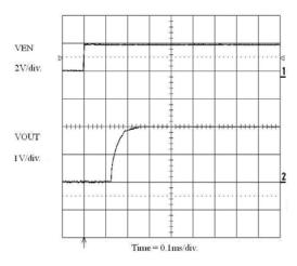
Figure 17. Enable Turn-On (1000 mA Load)
