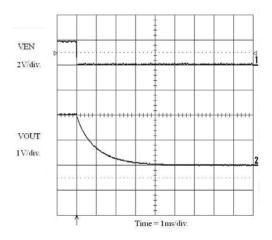
Figure 16. Enable Turn-Off (1 mA Load)
