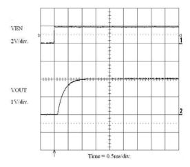
Figure 19. Enable Turn-On (1 mA Load) CBYP = 470 pF
