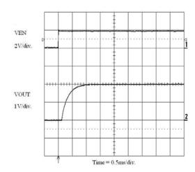
Figure 20. Enable Turn-On (1000 mA Load) CBYP = 470 pF
