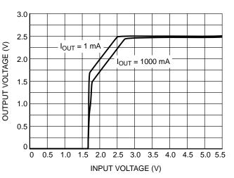
Figure 7. Dropout Voltage vs. Load Current
