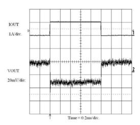
Figure 23. Load Transient Response (1 mA to 1000 mA)
