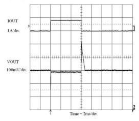
Figure 26. Load Transient Response (1 mA to 800 mA) ( $V_{OUT}$  = 0.8 V and  $V_{IN}$  = 1.8 V)
