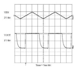
Figure 21. Slow Enable Operation (1 mA Load)
