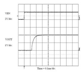
Figure 15. Enable Turn-On (1 mA Load)
