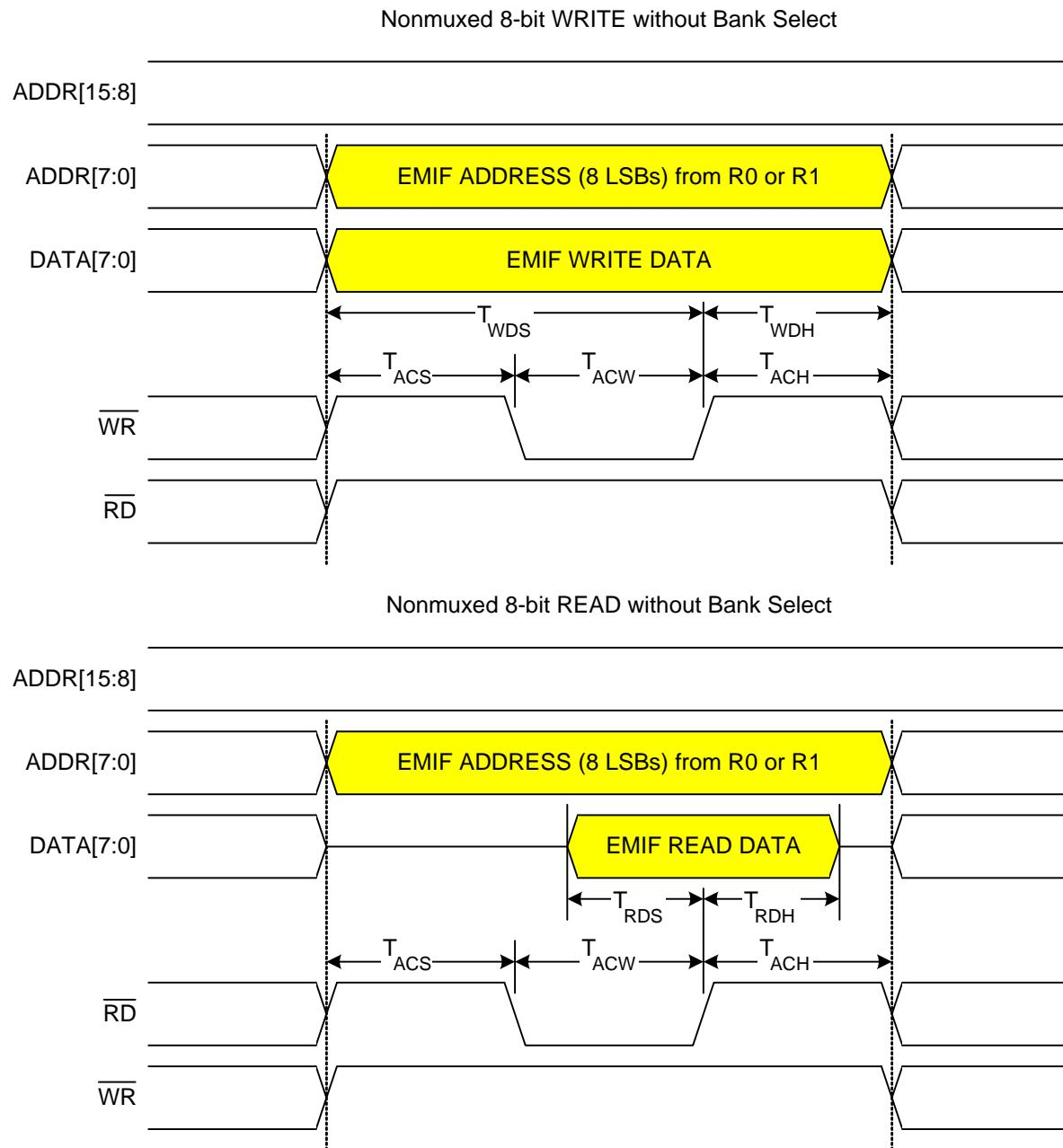
Figure 10.5. Non-multiplexed 8-bit MOVX without Bank Select Timing
