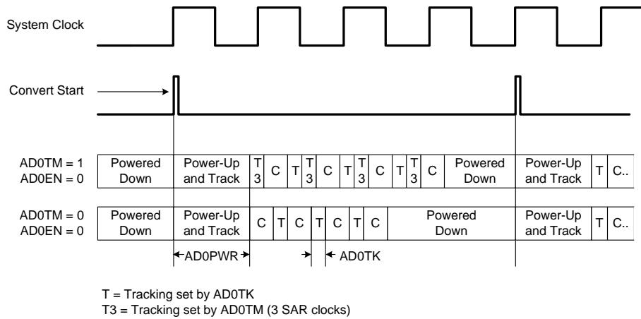
**Figure 5.3. Burst Mode Tracking Example with Repeat Count Set to 4**
