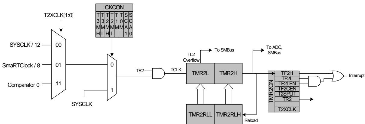
Figure 32.4. Timer 2 16-Bit Mode Block Diagram
