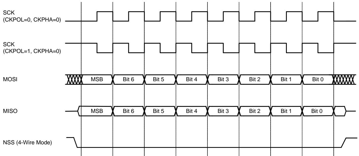
**Figure 30.6. Slave Mode Data/Clock Timing (CKPHA = 0)**
