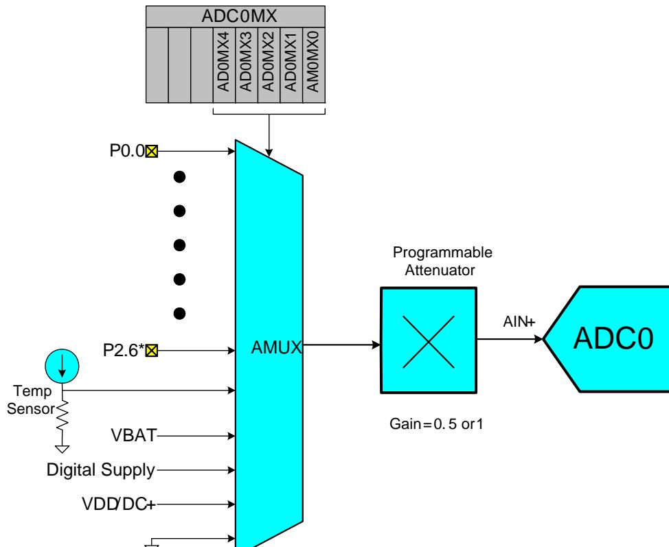
**Figure 1.14. ADC0 Multiplexer Block Diagram**
