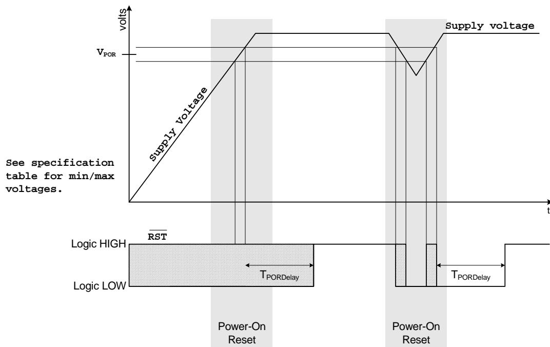
Figure 22.2. Power-On Reset Timing Diagram
