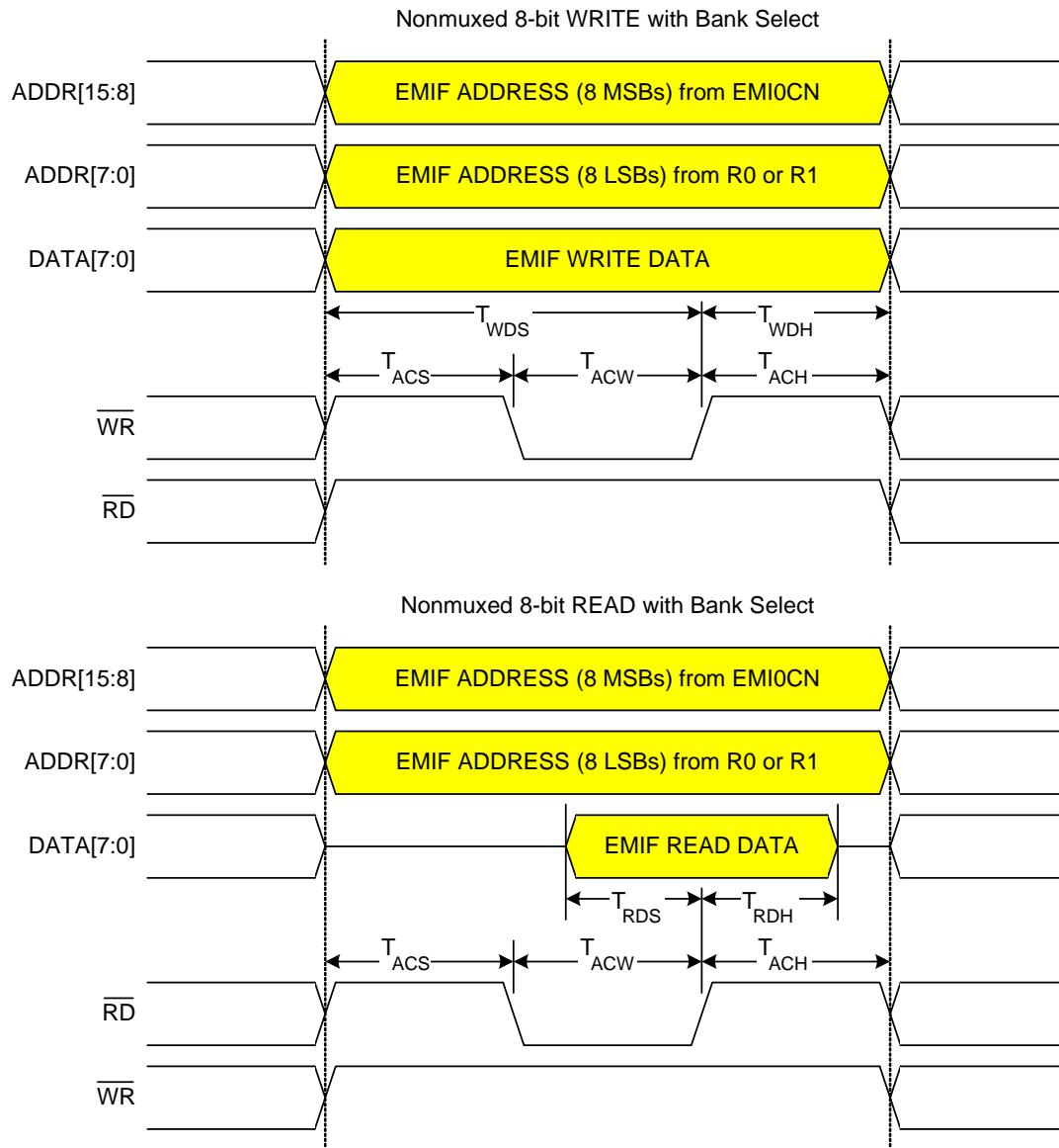
**Figure 10.6. Non-multiplexed 8-bit MOVX with Bank Select Timing**
