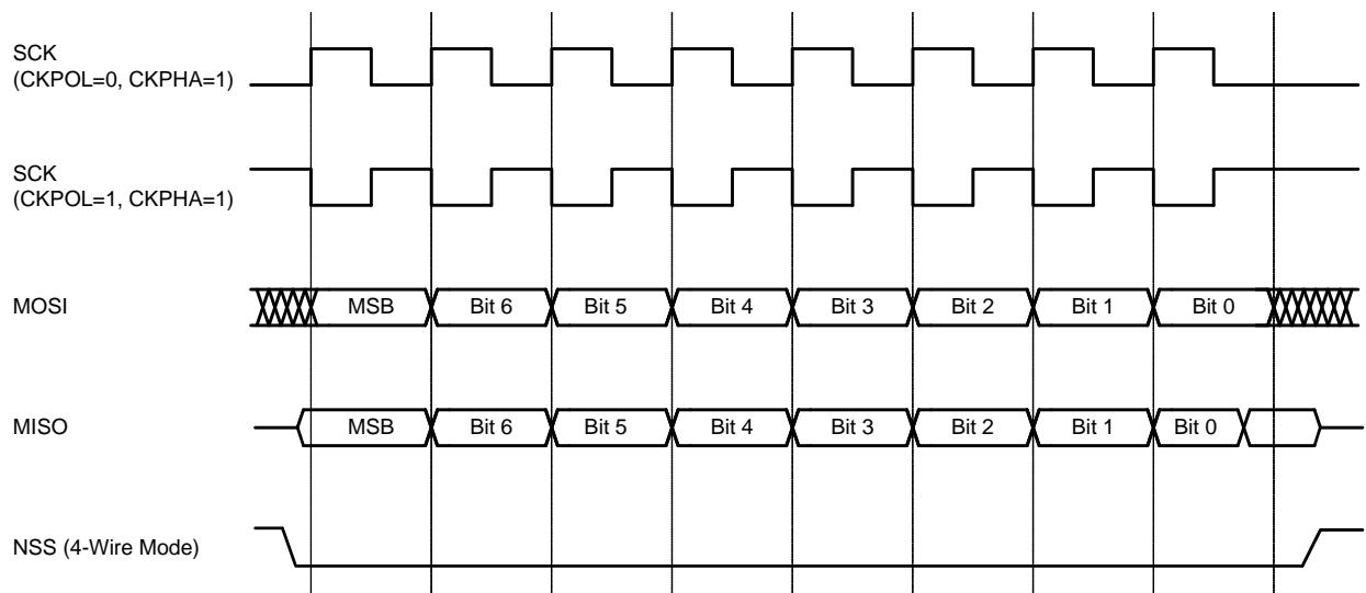
**Figure 31.7. Slave Mode Data/Clock Timing (CKPHA = 1)**
