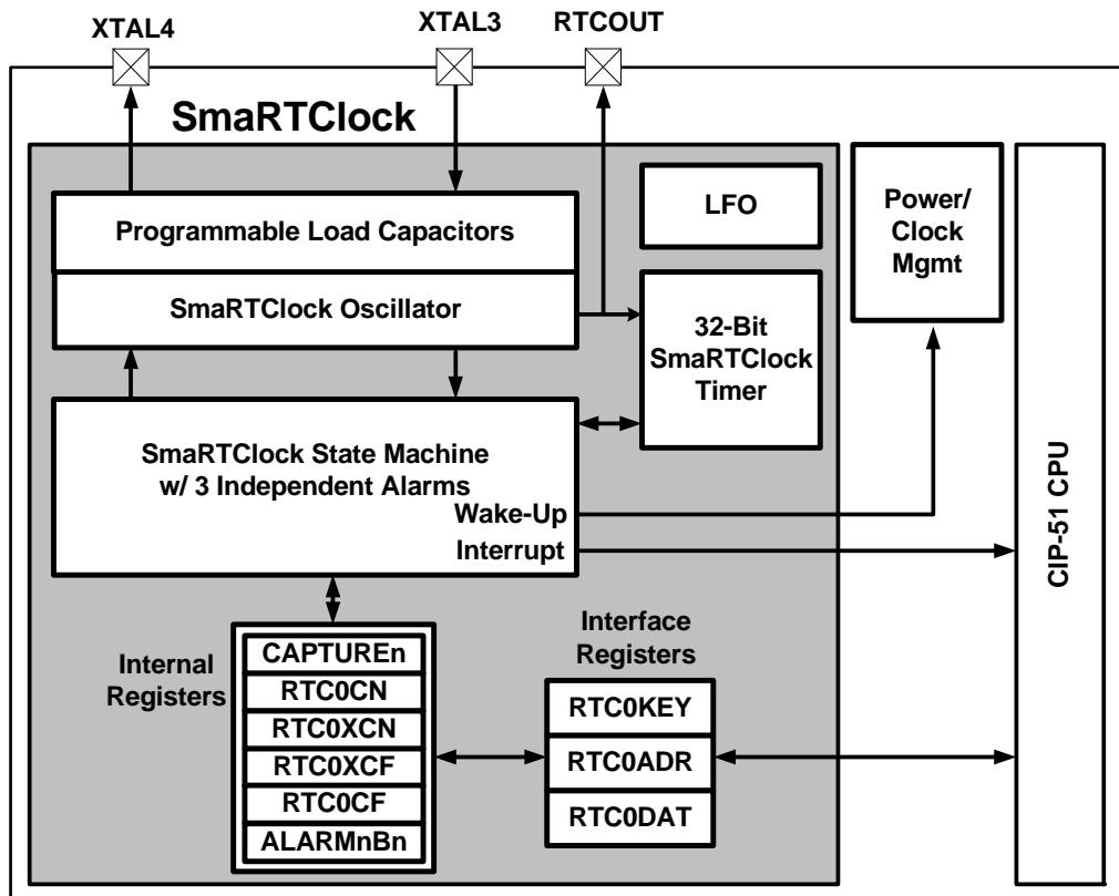
Figure 24.1. SmaRTClock Block Diagram
