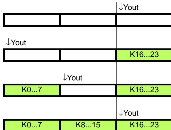
When using a 256-bit key, the DMA0NSZ can be set to 32 and the DMA0NAOL set to 16. This will place the last 16 bytes of the 256-bit key in the desired location as shown in Table 14.3. Enabling the WRAP bit in DMA0NMD will reset the DMA0NAO value after byte 31. Then the DMA0NZ can be set to 16 for the remaining sixteen bytes.
