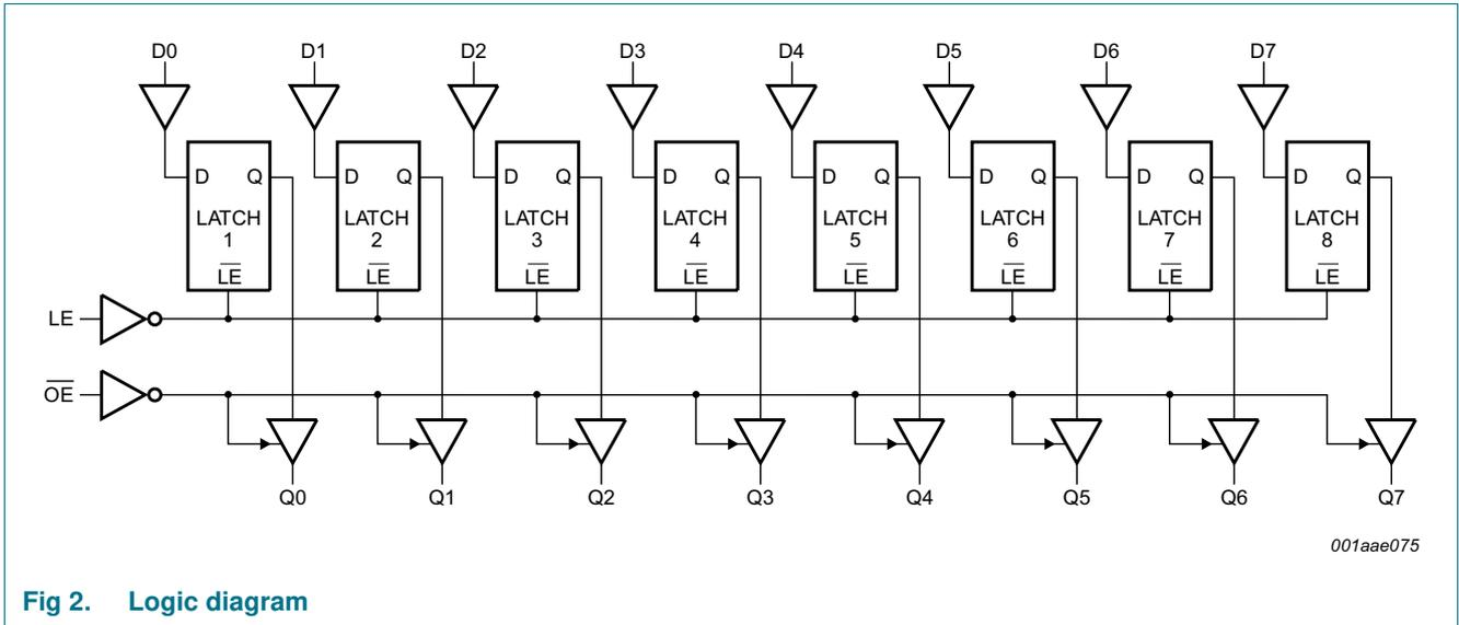
Fig 2. Logic diagram
