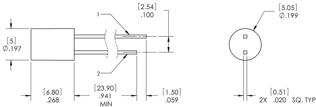
1 ANODE 2 CATHODE DIMENSIONS ARE IN INCHES AND [MILLIMETERS].
