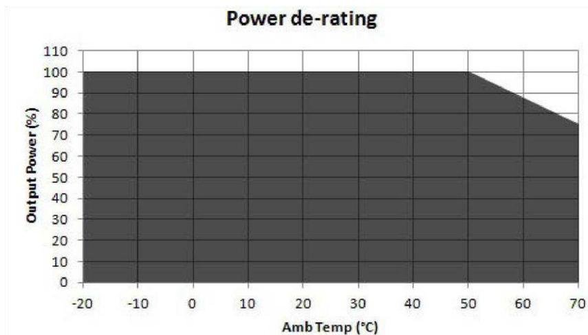
Figure 1. Derating Curve
