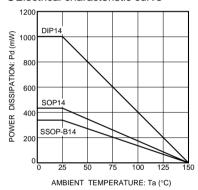
Fig.3 Power dissipation vs. Ta
