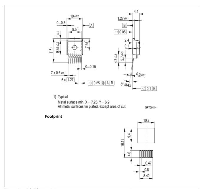
Figure 16 PG-TO263-7-1 (Plastic Green Transistor Single Outline Package)
