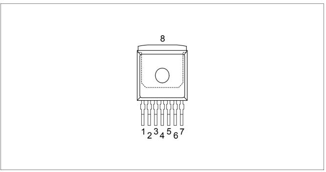
Figure 3 Pin Assignment BTN7933B (top view)
