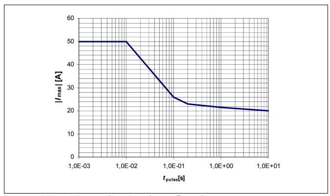
Figure 4 BTN7933B Maximum Single Pulse Current ( $T_c < 85^{\circ}C$ )
