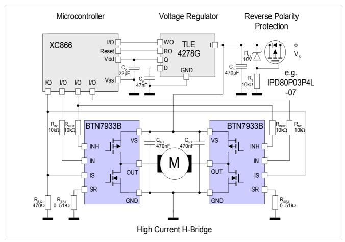
Figure 14 Application Example: H-Bridge with two BTN7933B
