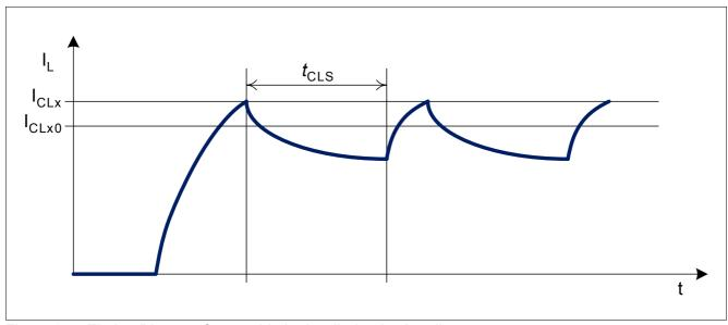
Figure 9 Timing Diagram Current Limitation (Inductive Load)
