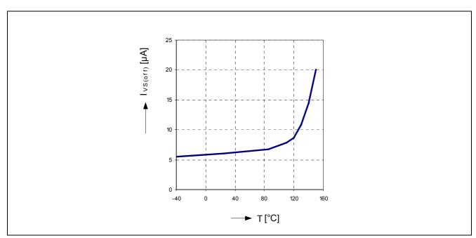
Figure 5 Typical Quiescent Current vs. Junction Temperature
