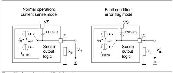
Figure 12 Sense Current and Fault Current
