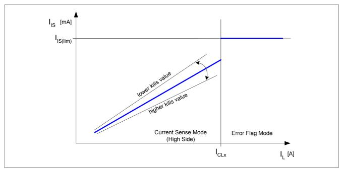
Figure 13 Sense Current vs. Load Current
