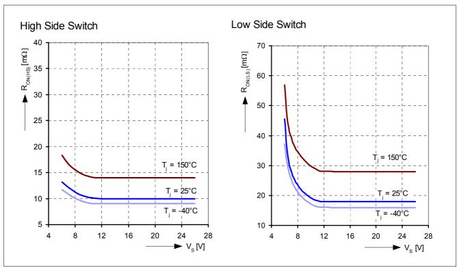
Figure 6 Typical ON State Resistance vs. Supply Voltage
