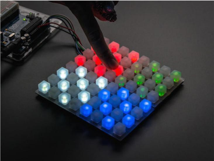
Four *Trellises* are combined to make a single large **8x8 matrix** for UNTZtrument. The HELLA UNTZtrument has *eight* *Trellises* in a 16x8 matrix!
