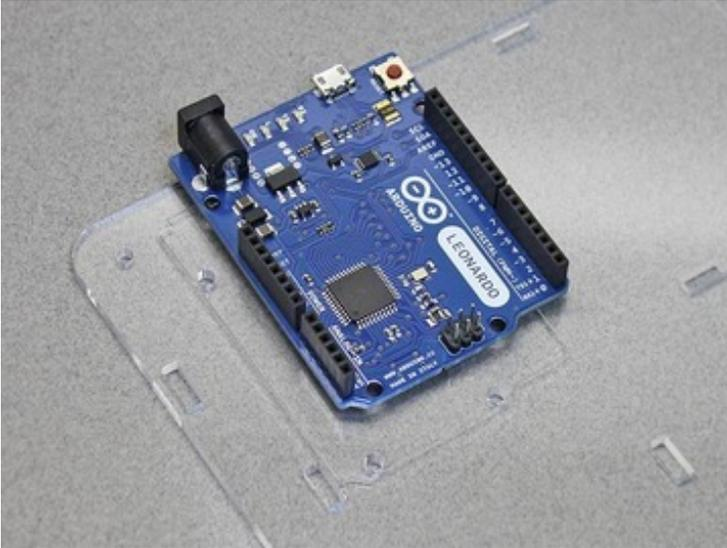
This piece has the Arduino footprint scored on one face. This helps identify the top surface.
