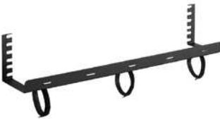
This zero-rack-unit Tie-Down Rack mounts horizontally on 19-in. racks. It takes up minimum space yet effectively controls and separates cable runs. Made of steel with RAL 9005 black polyester powder paint finish. Includes slots for cable wraps. Each rack includes 10 black 8-in. (203-mm) VELCRO® cable wraps. Mounting hardware included.
