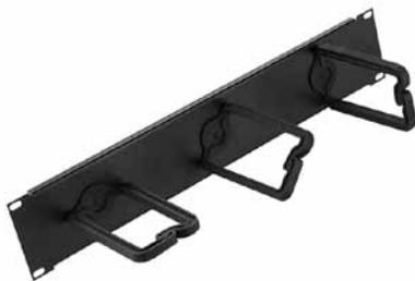
Mounts horizontally on 19-in. racks. Allows grouping vertical cable runs. D-Rings rotate on bracket for easy cable positioning; snap open for easy access for cable updates, yet latch securely. Back plate made of steel with RAL 9005 black polyester powder paint finish; D-Rings are black plastic. Mounting hardware included.
