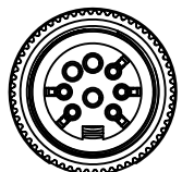
AISG 8-pin female interface with 5 loaded contacts
