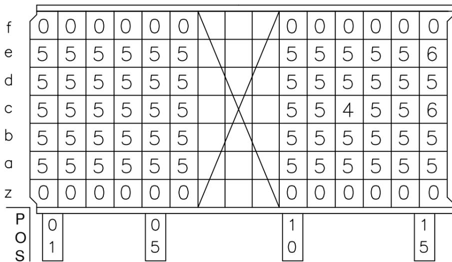
LOADED CONNECTOR ASSEMBLY (FOR EXAMPLE)
