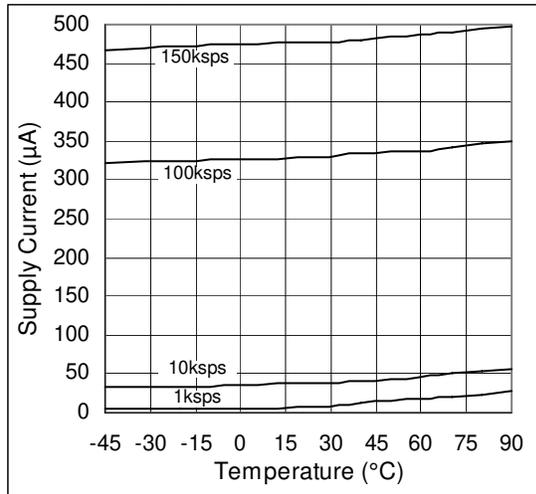
Figure 9. Supply Current vs. Temperature,  $V_{DD} = 3V$
