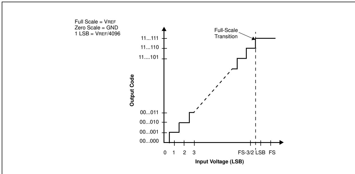
Figure 22. AS1524 Bipolar Transfer Function
