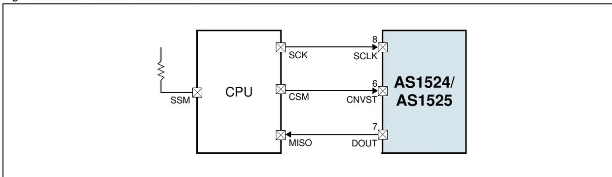
Figure 27. QSPI Serial Interface Timing (CPOL = CPHA = 0)
