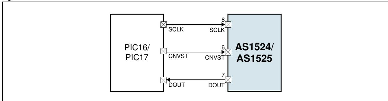
In SPI mode, the PIC16/PIC17 processor allow 8 bits of data to be synchronously transmitted and received simultaneously. Two consecutive 8-bit readings (see Figure 29) are necessary to obtain the entire 12-bit result from the AS1524/AS1525. DOUT data transitions on the serial clock's falling edge and is clocked into the processor on SCLK's rising edge.
